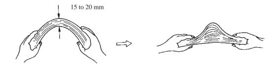
4 Take documents to be placed in the ADF paper chute. The thickness of the documents to be placed in the ADF paper chute is limited depending on the size of the documents as follows:
